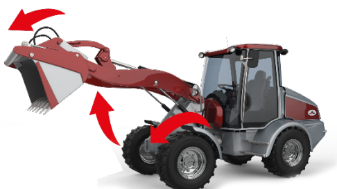
Fig. 2 – Energy savings with combined use of Walvoil ALS and EPX Hydraulic Digital Solutions
